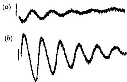
Figure 1. NMR signals obtained at 0.04 T from a 2.5 mM aqueous solution of TEMPOL: (a) without EPR irradiation; (b) with EPR irradiation at 1.12 GHz (same vertical scale as (a)).
